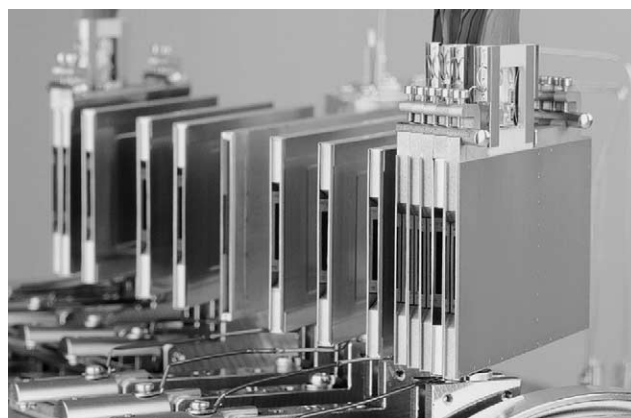
Fig. 14. Multiple collector array from the Finnigan TRITON and NEPTUNE. Miniaturized ion counters identical in size to Faraday detectors are mounted on the high mass side (for U) and low mass side (for Pb). Connections to the miniaturized ion counters are completely independent from the Faraday cup signal lines protecting the integrity of the signals.
